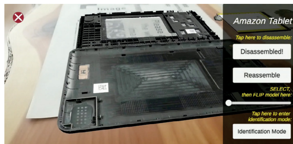
Fig. 6. MIT-developed augmented reality (AR) app enables measurement and disassembly of 3D photo-realistic reconstructions of products such as a consumer electronics tablet.
